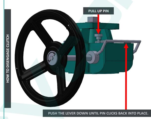
WHEN USING SPRING RETURN ACTUATORS, IT IS CRUCIAL TO ENSURE THAT THE ACTUATOR IS RETURNED TO ITS RELAXED SPRING POSITION REFORE DISENGAGING THE CLUTCH, THIS PRECAUTION HELPS MAINTAIN PROPER FUNCTIONALITY AND PREVENTS ANY
