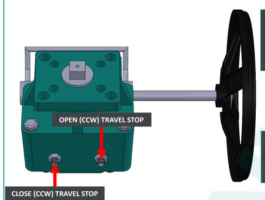
Travel Stop Nuts (Loosen Counterclockwise to Adjust Stop, then Re-tighten):
